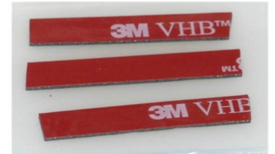
3M VHB Tape to secure wires.
